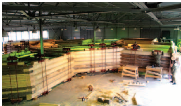
Fig. 14. The church basement framework under “Loading simulation” test
