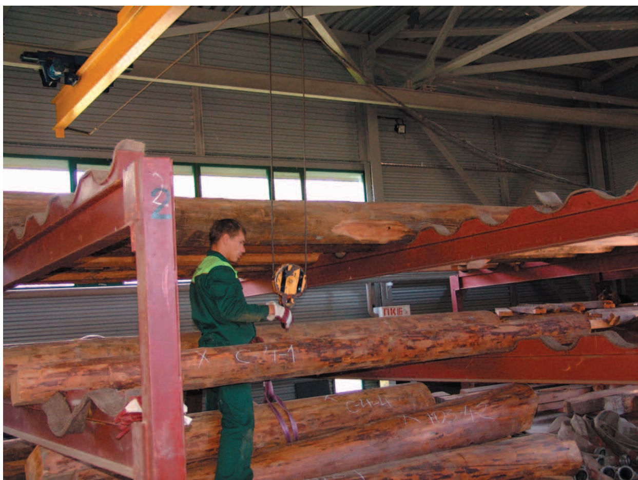
Fig. 10. Stacking of logs on stacks equipped with felt-covered cradles in the Restoration Complex
