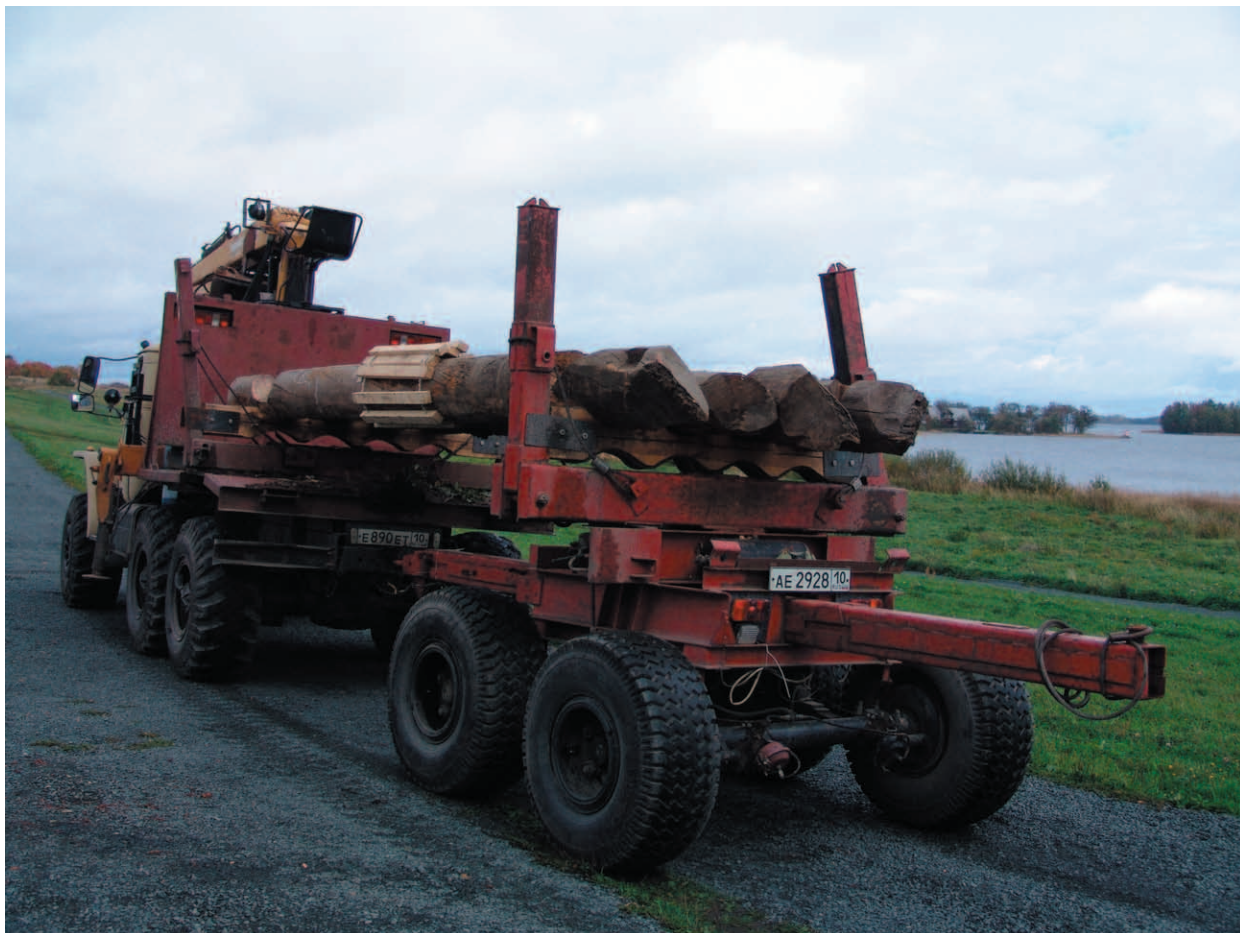
Fig. 9. Transportation of a small number of logs by specially equipped timber lorry
