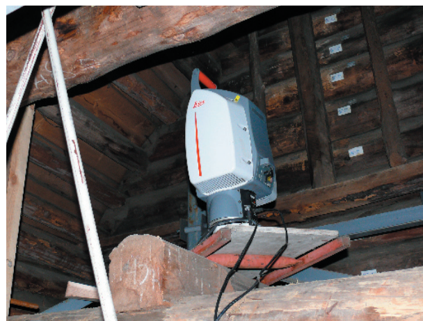
Fig. 4. 3d-scanning of the interior of the Church of the Transfiguration
